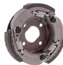
Clutch Malossi Fly Clutch d=107 Yamaha Aerox / BW's
