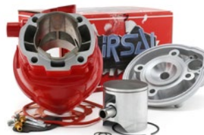
Cylinder Airsal Xtreme 88cc stroke=45mm Yamaha Aerox /
