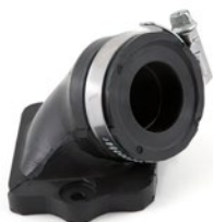
Intake Manifold Barikit 12-21mm Piaggio NRG / Typhoon
