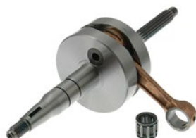
Crankshaft Malossi MHR RHQ piston pin=12mm Yamaha Aerox
