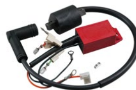
CDI Top Performances Piaggio, derestricted, variable ignition Type: //Ignition coil & CDI Brand: TOP PERFORMANCES Art. No.: T9924880
