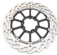
Brake Disc floating Moto Master Supermoto Racing 320mm TM
